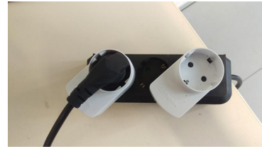
Figure 5.3: Plugwise energy sensors
