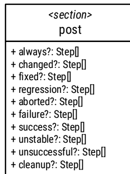
Figure 5.3: Class diagram of the post section in StalkCD
