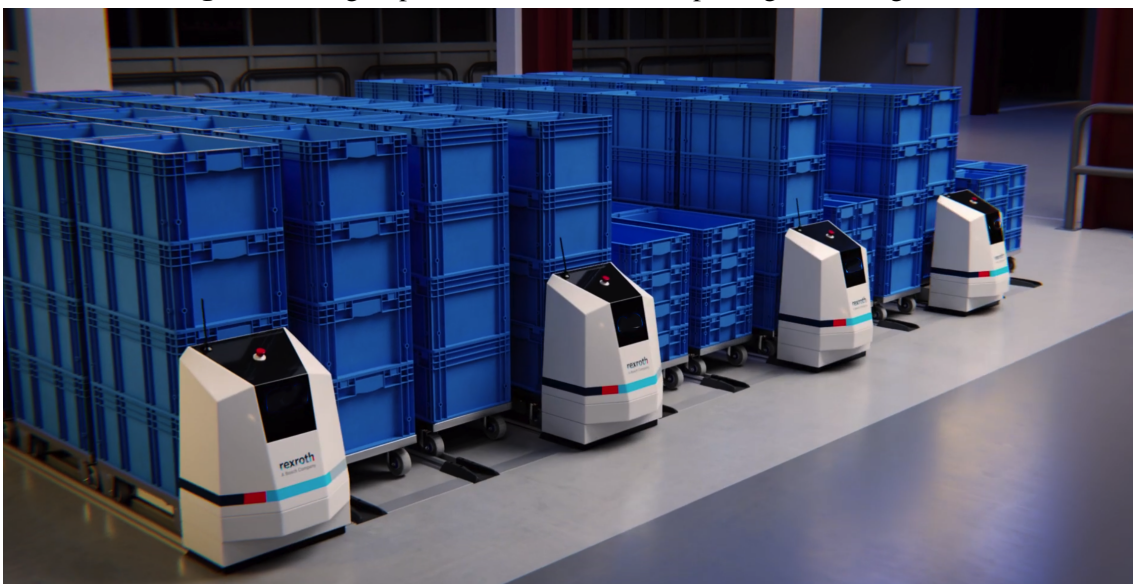
Figure 1.4: A group of Active Shuttles transporting boxes of goods.
