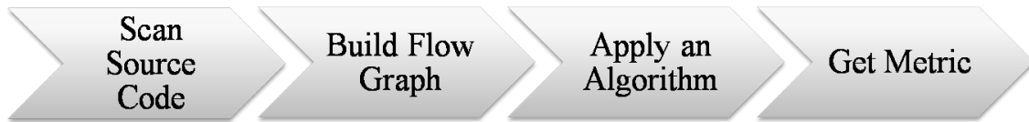
Figure 3.2: Process of Structural Analysis Model
