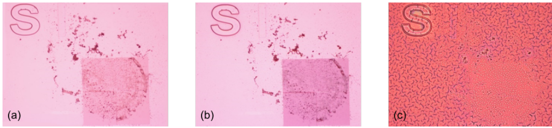
Figure 5.11 SOG spin-coated on meander structure: (a) Image after spin-coating; (b) Image after heating 2 min at 200 degree; (c) Image after heating 5 min at 200 degree.
