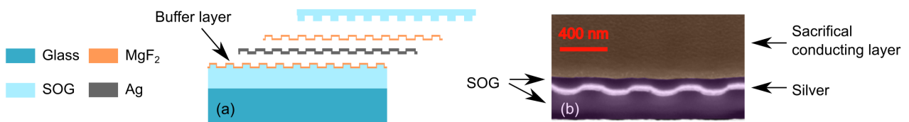
Figure 5.17 (a) Fabrication procedure of one layer silver meander structure; (b) Cross-sectional SEM image of a fabricated single layer meander structure.
