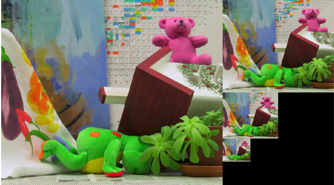
Figure 2.3: Image pyramid of 4 levels with the down-sampling factor \eta = 0.5 . Image is from the Teddy sequence of the Middlebury dataset [BSL11].
