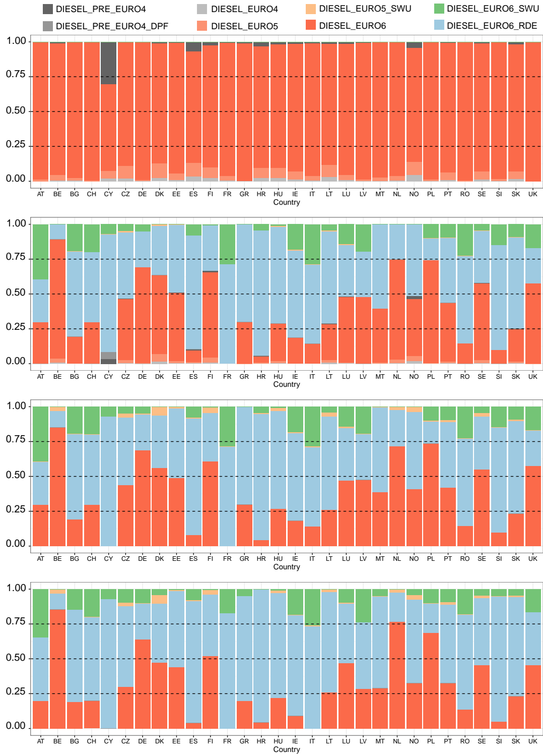
Figure 6-1: Technology distribution within fleet of diesel-fuelled cars and vans in urban areas across Europe. The lower two scenarios have LEZs in place. The figure shows technology distribution in the reference case (top), social-welfare optimum (2nd from top), and with NOx reduction goals of 25% (3rd from top) and 75% (bottom) as a result of taking different measures.
