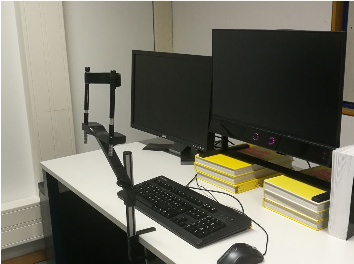
Figure 4.2: Setup of the study with the headrest and eye tracker.
