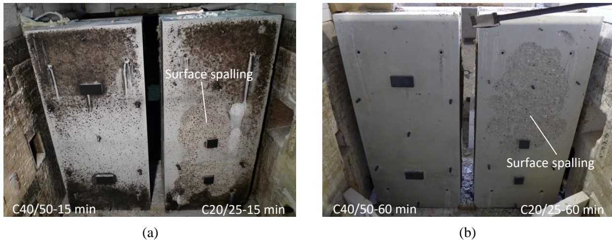
Figure 5.6 Fire effect on the concrete specimens after (a) 15 min and (b) 60 min of ISO 834 fire.
