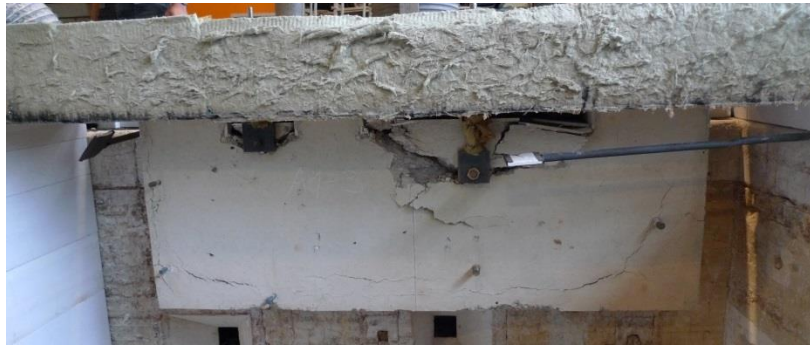
Figure 4.7 Specimen after fire exposure up to 90 min.
