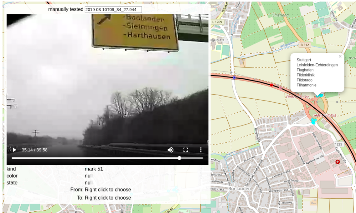
Figure 3.1: User Interface to manually evaluate the destination sign coverage in OpenStreetMap. The black line is the driving route of the car as derived from the recorded GPS locations. The cyan dots are the destination signs that are tagged in OpenStreetMap. Clicking on them reveals their destinations in a bubble. The blue dots are the markers that were made when a sign was seen while driving. The pink dot is the currently selected marker. The red dot is the GPS location closest to the currently seen frame in the video. In this scenario the complete information of the real world sign seen in the video is correctly tagged in OpenStreetMap. (Map credits: [OSM])
