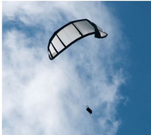
Figure 2.1.: AWE system consisting of a leading edge inflatable kite, bridle lines and a kite control unit [33]
