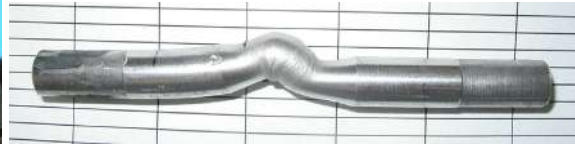
Sample bent in compression phase during push-pull deformation controlled test
