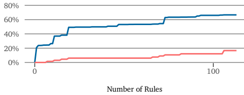
Figure 7.5: Influence of the number of selected rules (LANG project). The number of rules influences the — proportion of low-fault-risk methods and the — share of faulty methods in LFR out of all faulty methods.
