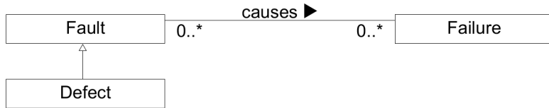
Figure 2.3: Relation between fault, defect, and failure.
