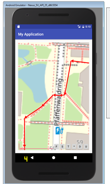
Figure 4.3: multiple arrows drawn using the same code with canvas rotation and translation
