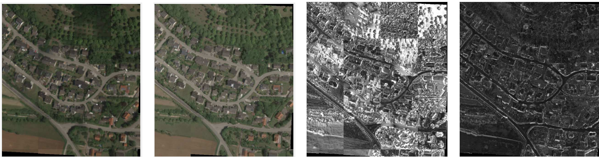
(a) RGB mosaic of Greding reflectance data (b) RGB mosaic of Greding1_ref and NFNalign Greding2_rad & Greding3_rad (c) RMSE mosaic of Greding reflectance data, scaled to RMSE values \in [0, 400] . (d) RMSE mosaic of Greding1_ref and NFNalign Greding2_rad & Greding3_rad, scaled to RMSE values \in [0, 400] .
