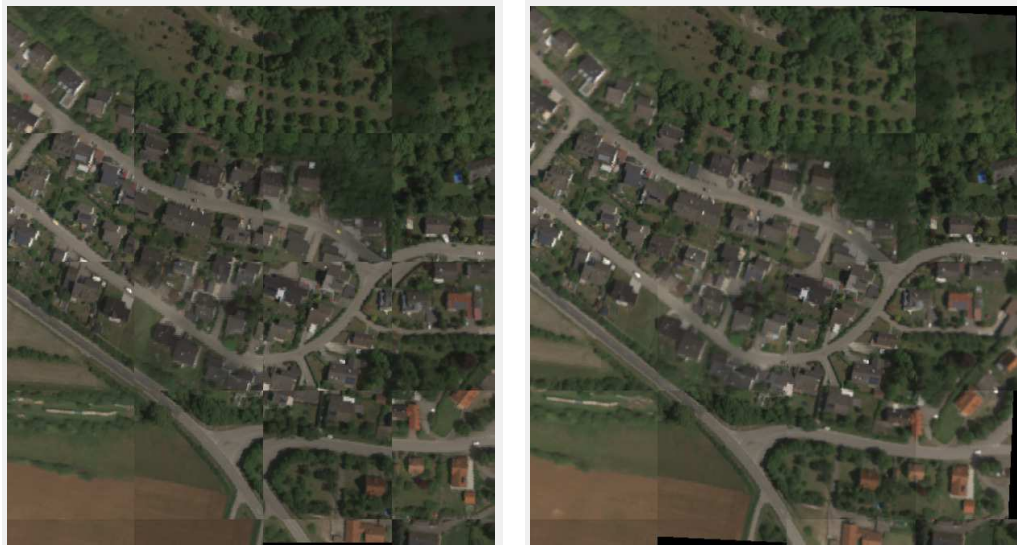
(a) Mosaic of georeferencing from raw GPS / INS data (b) Mosaic of georeferencing after GPS / INS post-processing, borsight correction and ECC maximization
