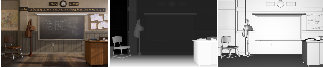
Figure 2.13: From left to right : Reference frame, color-coded depth visualization, shaded depth visualization.
