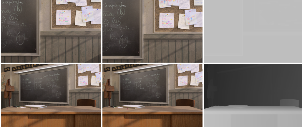
Figure 2.12: From left to right : Reference frame, subsequent frame, corresponding depth map. Top : Constant depth (first-order smoothness). Bottom : Affine depth (second-order smoothness).
