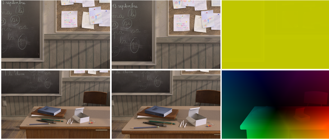
Figure 2.11: From left to right : Reference frame, subsequent frame, corresponding motion field. Top : Constant motion (first-order smoothness). Bottom : Affine motion (second-order smoothness).
