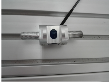
Figure 4.30: Force sensor KM30z with forces up to 1kN
