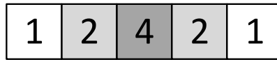
Figure 4.6: Exemplary one-dimensional weighting stamp that influences all neighbors with distance \leq 2 . Source: [2] under CC BY-NC-ND 4.0
