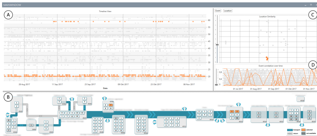
Figure 5.3: Experts can inspect the individual error event occurrences in the Timeline View (A). The Location View (B) provides information about the spatial distance between the selected stations. Stations that are similar regarding the patterns of reported events can be identified in the Location Projection View (C). To verify these correlations, the locations' correlation over time can be inspected in the Correlation View (D).
