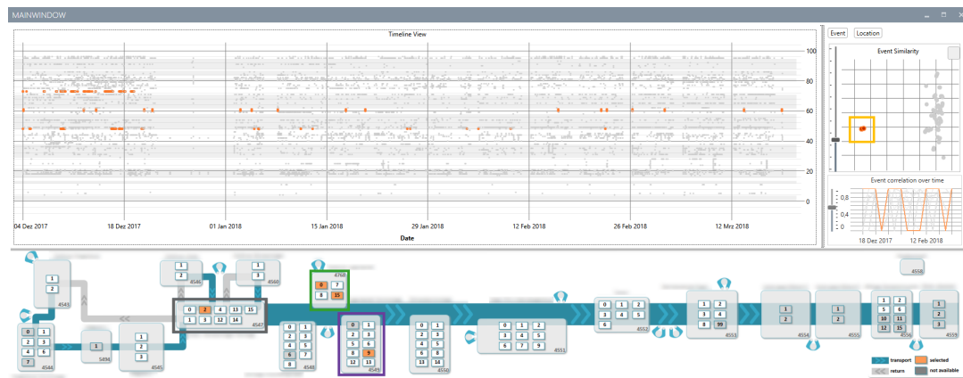
Figure 5.10: Through the selection of a clearly separated group of events types , it becomes apparent that there are error dependencies between the process steps 4547 , 4768 and 4549 . An expert can verify this hypothesis through the Correlation View and the Timeline View .
