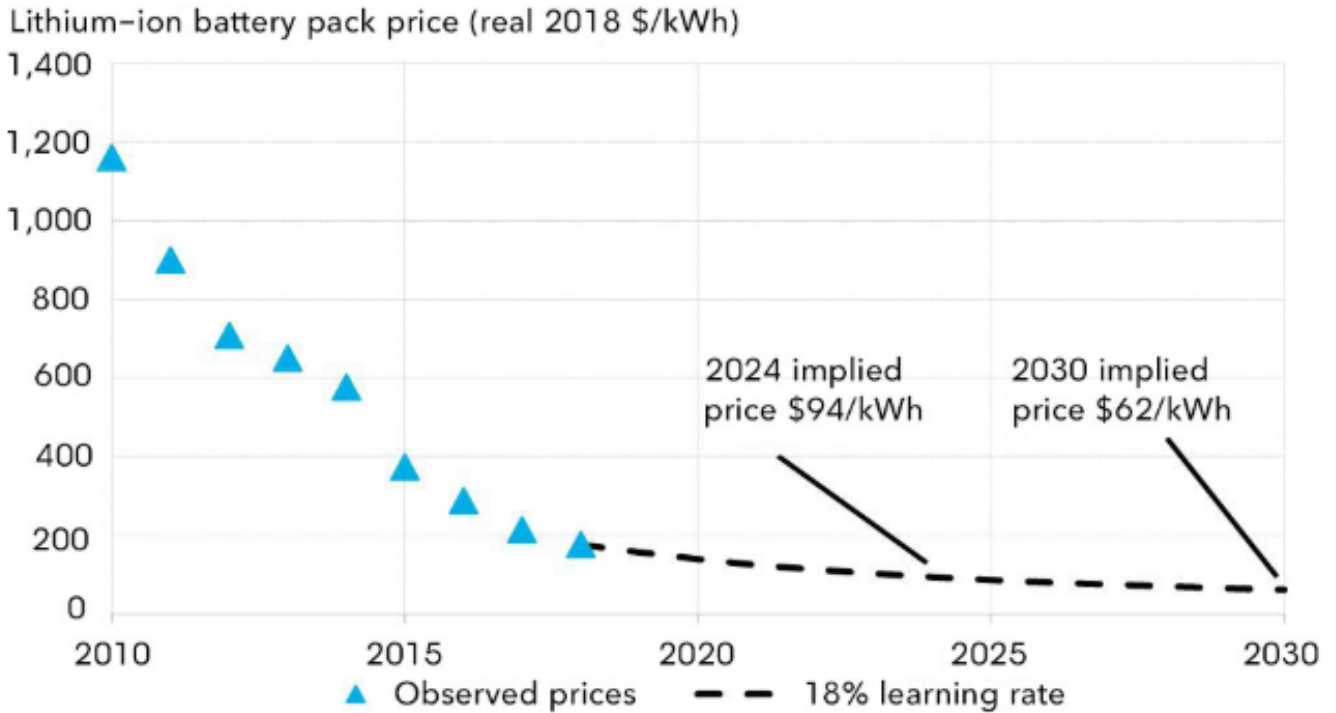
Figure 3: Another overview of past, current and future prices for batteries per kWh [13].
