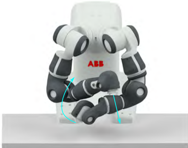
Figure 4.25: Dual-arm robot YuMi in crossed-arm configuration with motion commands causing deadlock indicated by blue arrows.
