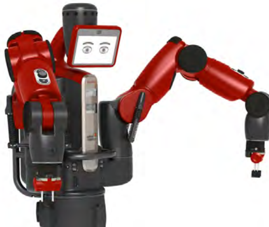
Figure 3.9: Rethink Robotics' dual-arm Baxter robot features a motion controller actively avoiding collisions between the arms.
