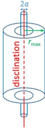
Figure 1.6: Schematic illustration of the parameters r_{\text{max}} which is the sample radius and a being the core of the disclination which is excluded from consideration.
