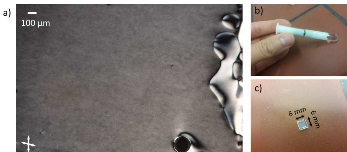
Figure 4.4: (a) Planar aligned LLC in a 100 \mu\text{m} thick cell. The center of the cell is without defects and therefore suited for dynamic light scattering measurements. (b) Sample holder for the cells manufactured by the workshop of the Institute of Physical Chemistry to put into the index matching fluid bath of the LS setup. (c) An example of a cell filled with 5CB and sealed with UV glue is shown.
