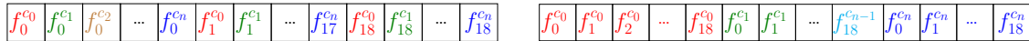
FIGURE 3.4 Struct-of-arrays-based storage scheme (streaming-optimized, left) compared to an array-of-structs-based storage scheme (collision-optimized, right) for a D3Q19 implementation of the LBM as it is used in ESPResSo. Colors encode the cell which the respective value is associated with.
