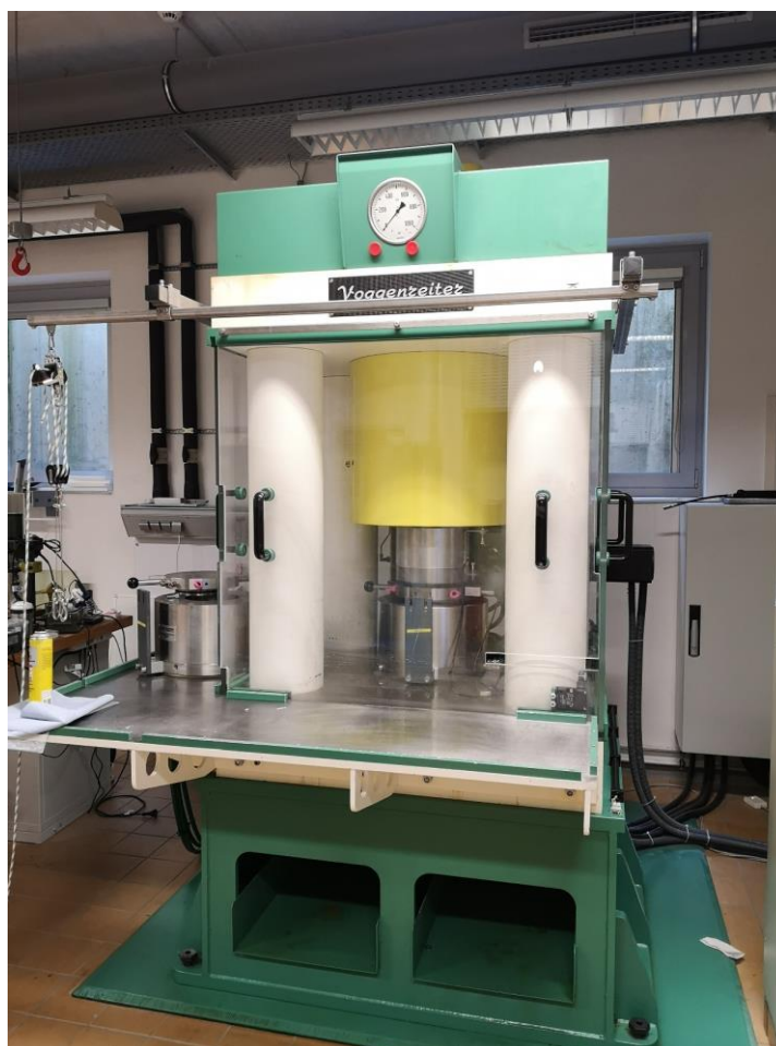
Figure 2.7. Voggenreiter press with a Walker-type multi-anvil module, located at the Max-Planck-Institut für Chemische Physik fester Stoffe, Dresden, Germany.
