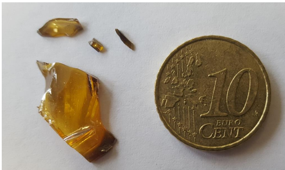
Figure 8.3. Large crystals of \text{Pb}_5\text{Ge}_3\text{O}_{11} produced by flux crystal growth.
