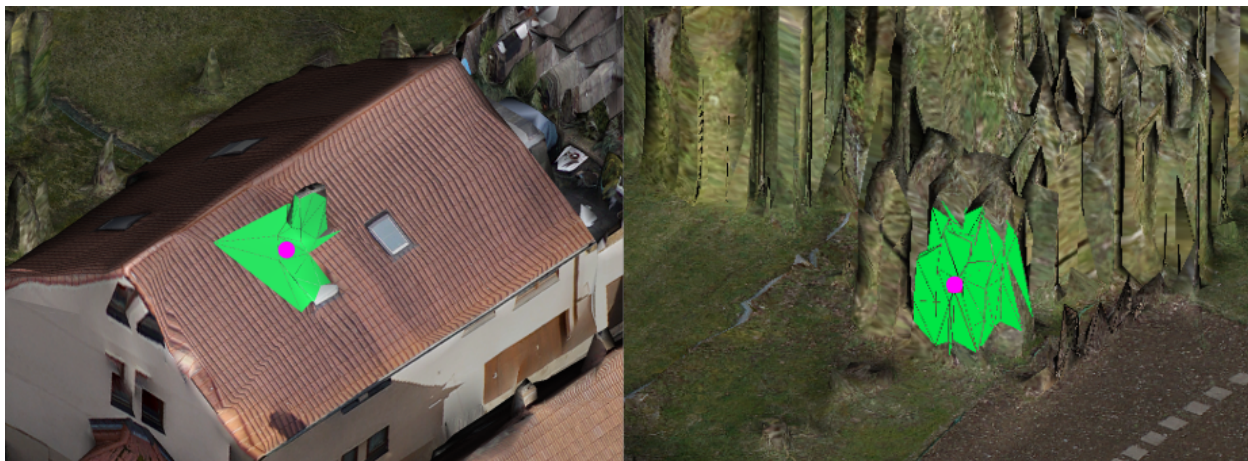
Figure 4.3: Submeshes of SPNH level 2 (radius 1.5 m) depicted in green. The pink dots mark the current face of interest, for which the SPNH-dependent feature calculation is performed.
