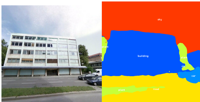
Figure 5.3: Input image and corresponding output from the FCN evaluation. The semantic class building is depicted in blue, sky in red, road in yellow, plant in green and car in bright blue, respectively.
