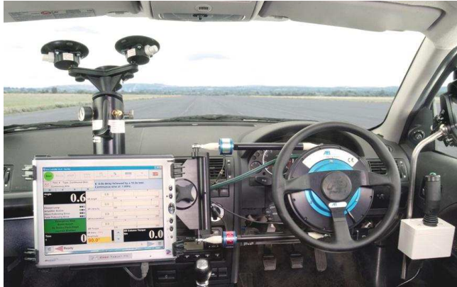
Figure 2.5.: Steering robot SR60 from Anthony Best Dynamics (Source: Anthony Best Dynamics, 2012) to validate steering wheel angle sensor
