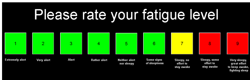
Figure 2.3.: MATLAB KSS input GUI for the driving simulator, similar to the touch screen in every vehicle
