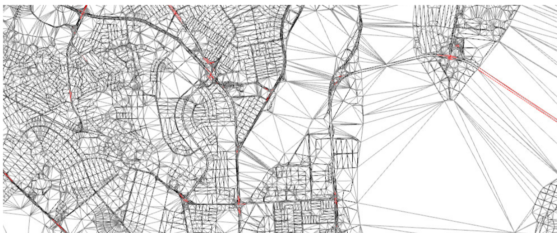
Figure 6.1: Spherical Delaunay triangulation (gray) constrained to contain all line segments (black) of streets in Ecuador and the intersection points of constraints (red).
