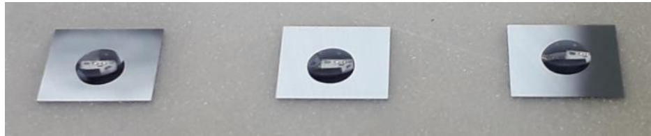
Figure 6. Epoxy adhesive is dispensed onto the backside of the chips after automated face-down placement on thermal release foil.
