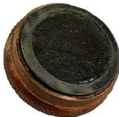
Figure 3-4. Thin-film sample prepared for the Oxford Phenix cryocooler (right) and the scheme of Bragg Brentano diffractometer (left). [3-4]
