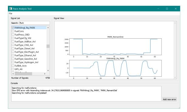
Figure 3.10: GUI of the Automated Trace Analysis Tool
