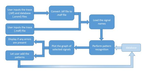
Figure 3.9: activity diagram of Automated Trace Analysis Tool
