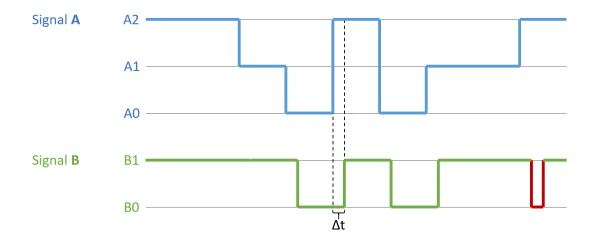
Figure 3.2: Discrete Signal Example with Latency
