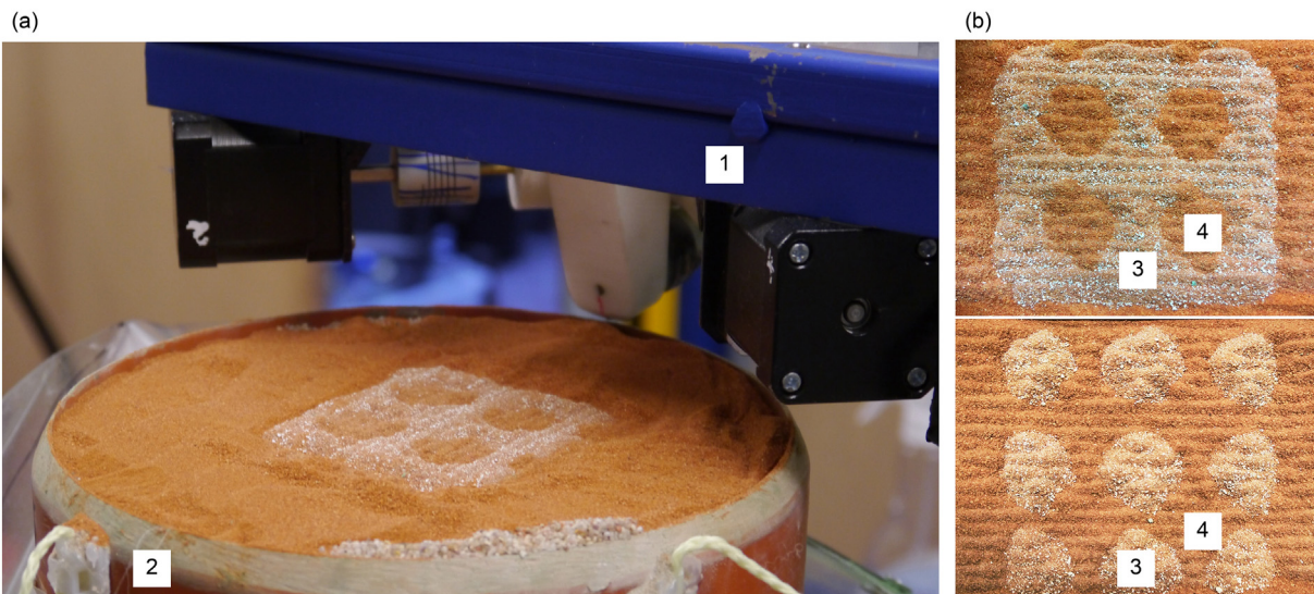
Fig. 12. 3D printing process: (a) Layer deposition by the print head - 1 on the print bed - 2; (b) Printed layers, where 3 - powder-sand mix (printed structure), 4 - pure sand (support structure).
