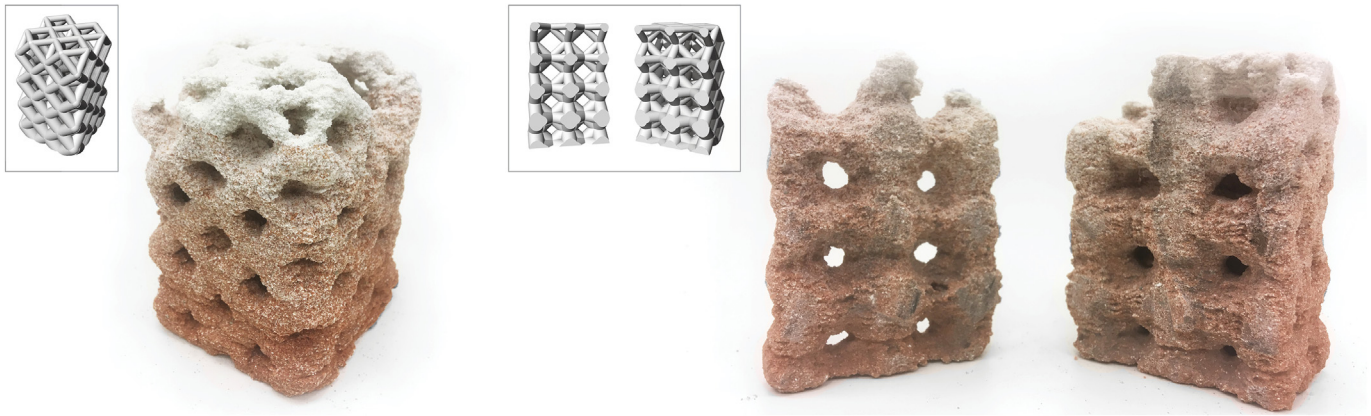
Fig. 13. Spatial structure produced with the developed additive manufacturing method: (a) Before cutting; (b) After cutting.
