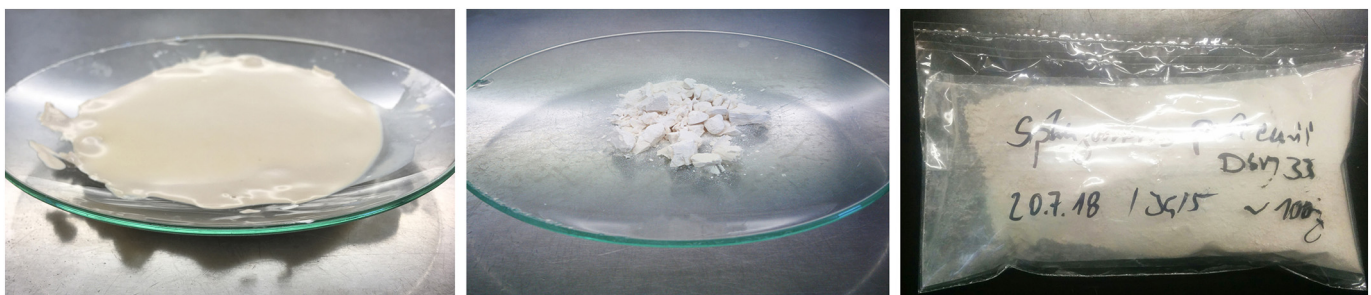
Fig. 1. Stages of calcium carbonate powder preparation: (a) Bioslurry before lyophilization; (b) Urease active calcium carbonate powder after lyophilization; (c) Vacuum-sealed powder.
