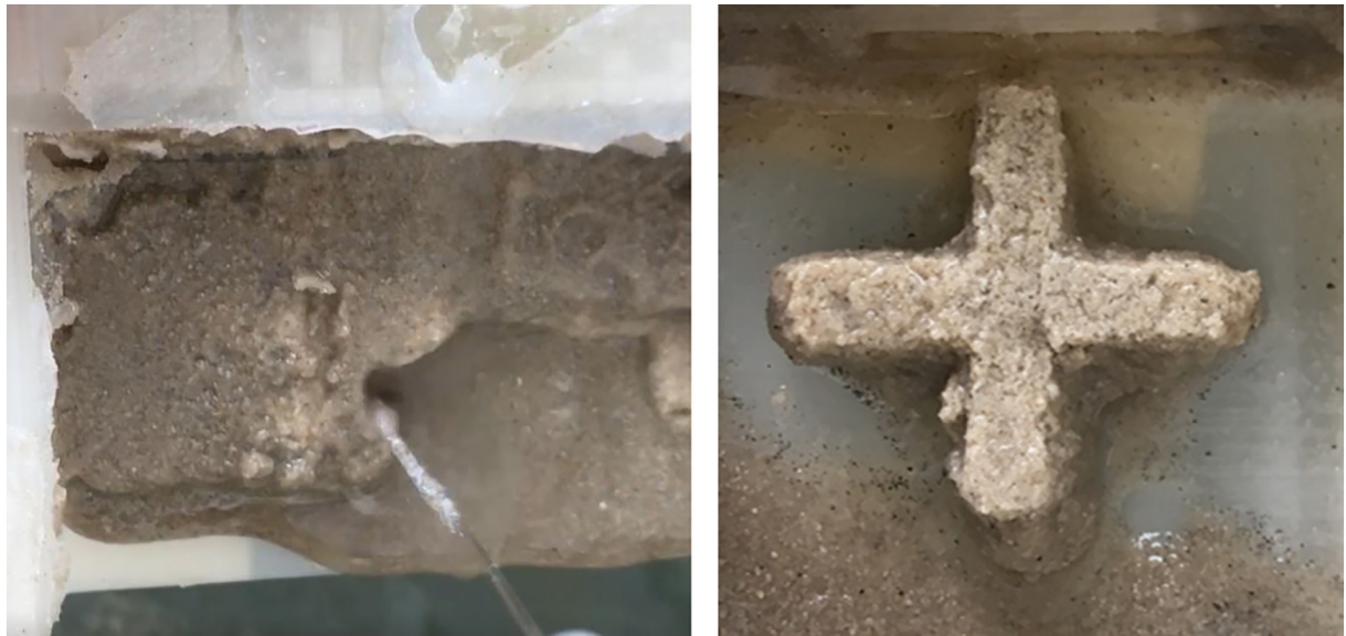
Fig. 10. Cementation of the urease active calcium carbonate powder-sand mix surrounded by pure sand: (a) Non-solidified sand being removed revealing a solidified structure; (b) Solidified structure.
