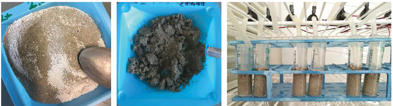
Fig. 3. Preparation of bio-cemented cylindrical samples: (a) Dry urease active calcium carbonate powder and sand; (b) Powder-sand mix moistened with the cementation solution; (c) Syringe bodies filled with the powder-sand mix during the treatment with cementation solutions.
