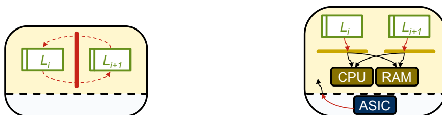
(a) Isolation of switch-local control processes (b) Fine-grained control resource control (RAM and CPU appropriation)
