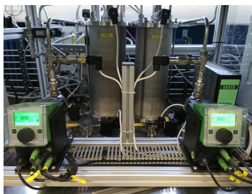
(b) Dosing pumps
