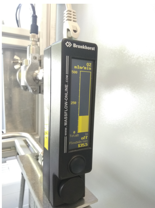
(c) Gas flow meter
