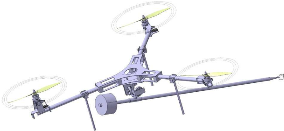
Figure 5.19: Concept sketch of an aircraft with a measurement boom mounted on an active gimbal.
