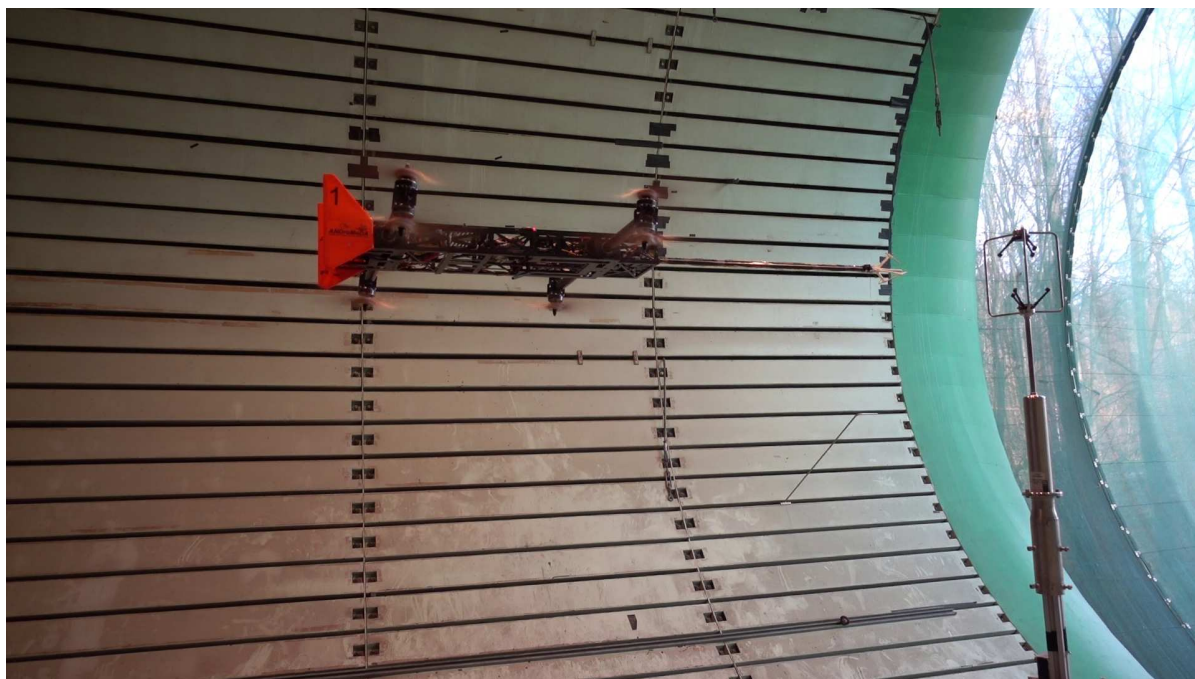
Figure 8.6: ANDroMeDA hovering inside the gust wind tunnel in close proximity to a sonic anemometer.
