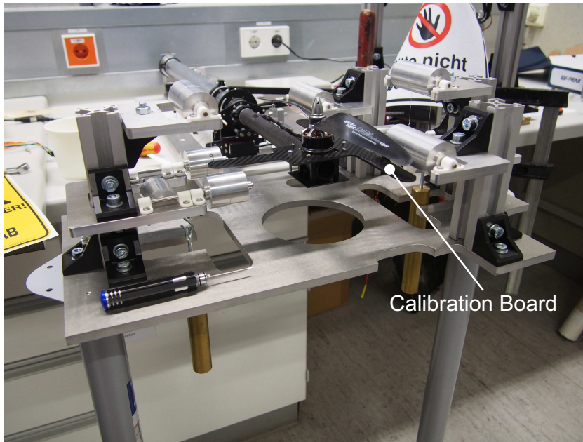
Figure A.39: Weights for -F_z calibration applied.
