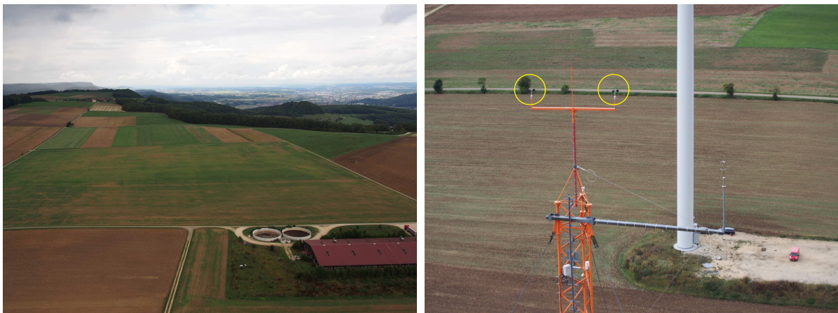
Figure 2.2: Left: View from above the met mast to the west. Right: Two cup anemometers mounted on top of the met mast.
