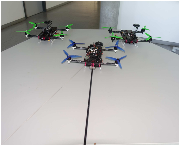
Figure 8.11: Automated group measurement control features can be tested with the three Baby ANDroMeDAs.
