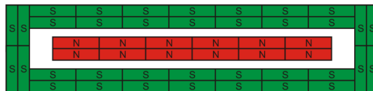
Figure 5.3: The array of 48 permanent cobalt-samarium magnets, arranged in a closed race track configuration, lying under the ECR vessel [4,6].
