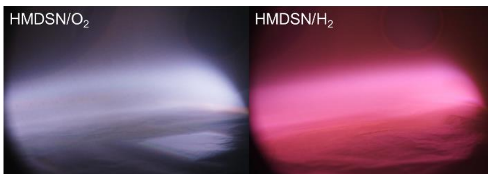
Figure 5.4: Plasmas seen from the side window port of the ECR vessel based on a HMDSN/oxygen (left) and a HMDSN/hydrogen (right) mixture.
