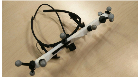
(b) Eye tracking goggles with removable 3D printed attachment for motion capture markers
