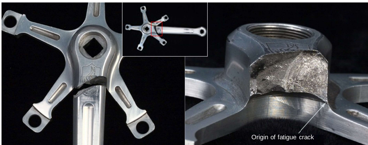
Figure 8: Fatigue failure in a bicycle pedal crank [05O].
