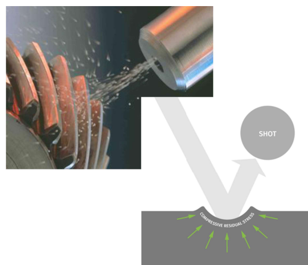
Figure 86: Shot-peening (SP) technique and its effect on the surface of a structural material [18T, 19P].
