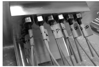
(b) Bottom side of the wall pressure module. The threads of the sensors are sealed with Loctite-222 and the reference pressure tubes are covered with silicone tubes.
