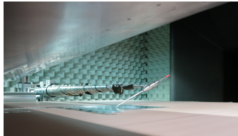
Fig. 6.1.7 View of the hot wire measurements close to Kulite sensor no. 4. The hot wire system is mounted on a traverse system with a long aluminum support cone.
