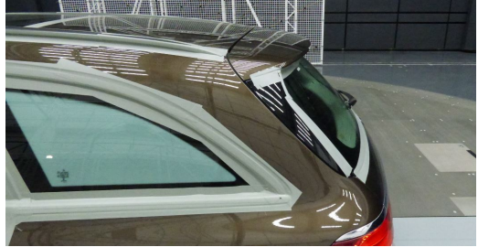
Fig. 1.2 Rear door gap of a Mercedes-Benz E-Class Estate (S213). Other visible openings or gaps are masked using cloth tape, the side windows are covered with heavy-weight mats inside the cabin.
