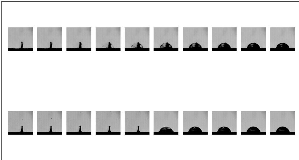
Figure 6.26: Interpolation of latent vectors of 3D AE: top - reconstructed interpolated vectors, bottom - corresponding real images.
