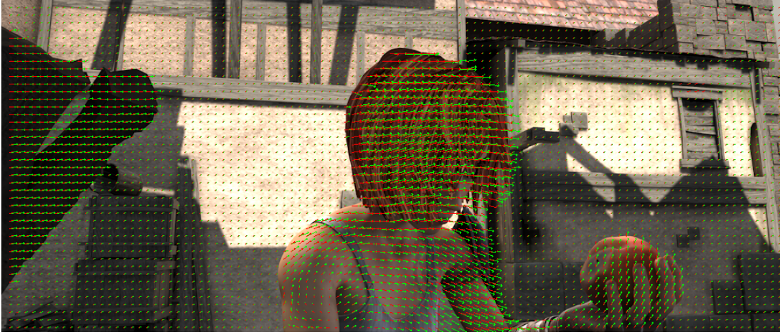
Figure 6.2: Baseline backward flows ( h = 4 ) for frame 5 of the alley_1 sequence. The first backward flow ( w_{t \rightarrow t-1} ) is denoted with green arrows while the second backward flow ( w_{t \rightarrow t-2} ) is denoted with red arrows. Refer to Appendix A.2 for a more in-depth example.
