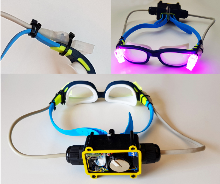
Figure 8.3: Final version of the prototype: the control button (right), the device working on the ACF mode (right) and a detail of the hardware (bottom).
