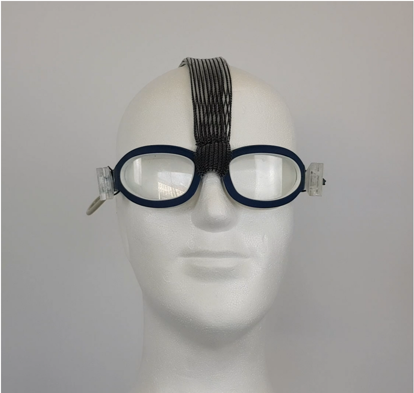
Figure 8.4: Final version of the prototype stabilized with a textile strap.
