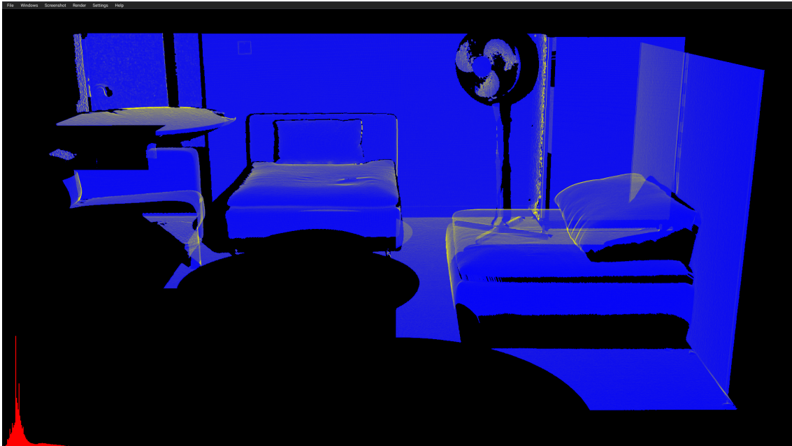
Figure 4.1: LiDAR dataset remodeling the interior of a room. A heatmap from blue to yellow encodes the number of points that are mapped to a single pixel. The values are linearly scaled from one point to 250 points per pixel. A histogram at the bottom further visualizes the point distribution among the pixels. With a number of 120131 most of the pixels contain 16 points. Planar areas perpendicular to the viewer build the densest regions.
