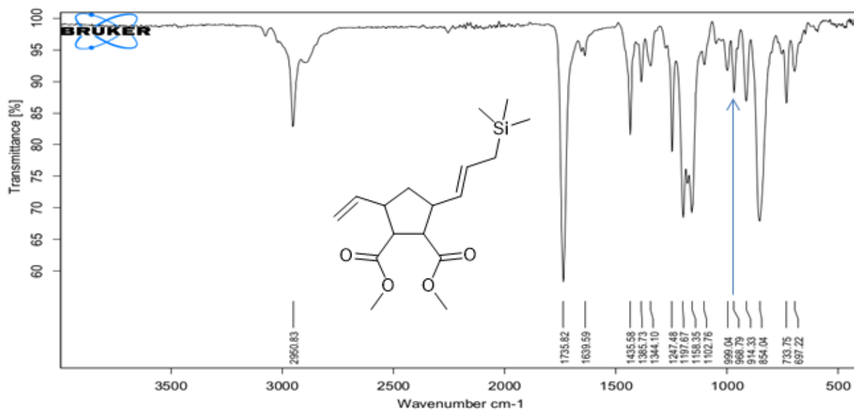
Figure 57. IR-spectrum of P3 . The characteristic peak for the trans -isomer is observed at 968.8 \text{cm}^{-1} .
