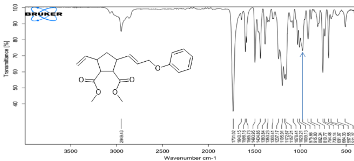
Figure 63. IR-spectrum of P5. The characteristic peak for the trans -isomer is observed at 975.7 cm -1 .
