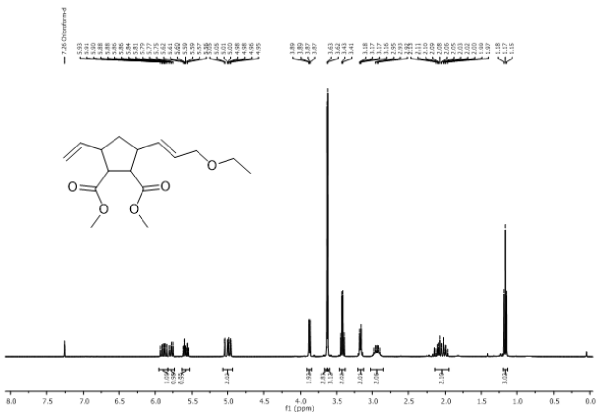
Figure 64. 1 H NMR spectrum of P6 (400 MHz, CDCl 3 ).
