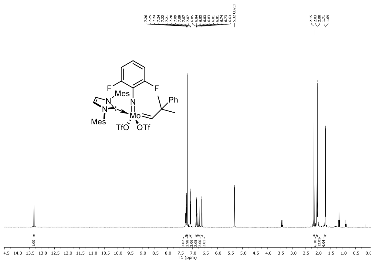
Figure 136. ^1\text{H} NMR spectrum of Mo-19 (400 MHz, \text{CD}_2\text{Cl}_2 ).
