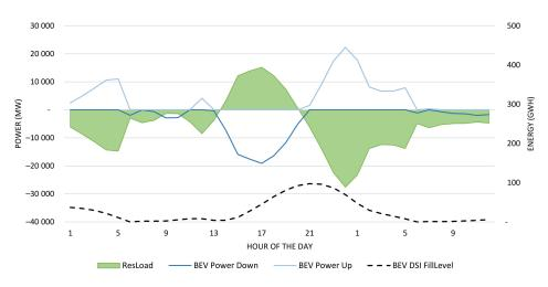
**Figure 6.** Use of *BEV-DSI* potential (PowerUp in light blue, PowerDown in blue) for 36 h to meet the residual load demands (ResLoad, green area). The corresponding fill level of the *DSI* storage is depicted in black dashes on the secondary axis.
