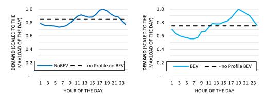
**Figure 11.** Exemplary depiction of the demand curves for the model runs without *BEV* (**left graph**) and with *BEV* demand (**right graph**) one time without profiles (black dashed lines) and with profiles (blue lines) for an exemplary day.
