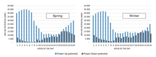
**Figure 5.** PowerUp (blue) and PowerDown (dark grey) flexibility potential of all *BEVs* for a typical Monday in spring and winter terms.
