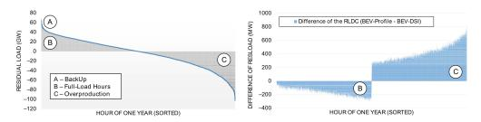
**Figure 12.** Residual load duration curve, congruent for the *BEV* scenarios (left graph), with the areas for the back-up need (**A**); full-load-hours (**B**) and overproduction (**C**). The right graph shows the resulting differences between the scenario without and with *BEV-DSI* concerning the FLH-reduction (**B**) and the overproduction (**C**). Concept of the figure based on [27].
