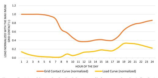
**Figure 2.** Depiction of the simulated realized charging profile for an exemplary day (yellow line), the maximum possible charging of all cars connected to the station (orange line), the maximum positive flexibility (blue arrow) and maximum negative flexibility (black arrow), normalized values.
