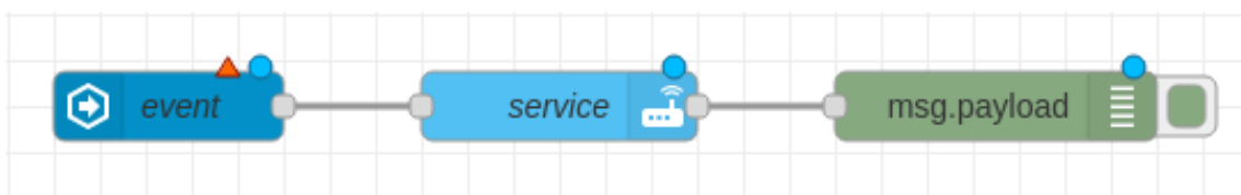
Figure 2.3: An Example Sequence of Nodes in Node-RED.
