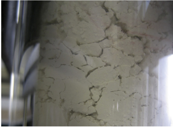
Figure 2.4: View on the reactor for direct charging after 4 reaction cycles shows agglomerates of \text{Ca}(\text{OH})_2 and preferential flow paths reprinted from [Roßkopf et al., 2014] 3
