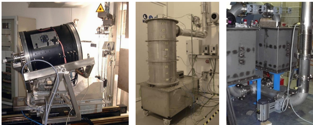
Figure 2.3: Selection of experimental setups of thermochemical energy storage reactors reported in the literature: Solar-heated rotary kiln (left), reprinted from [104], copyright 2012, with permission from Elsevier; packed bed TCS reactor (middle), reprinted from [93], copyright 2016, with permission from AIP Publishing; pilot-scale TCS unit consisting of \text{Co}_3\text{O}_4 coated cordierite honeycomb structures (right), reprinted from [140], copyright 2017, with permission from Elsevier.
