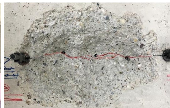
c) Figure 8.17. a) Load-displacement curves of test series G61 and G62R, b) Anchor force-time curve of test G62R-1, c) breakout body of one representative test of series G61, d) failure pattern of one representative test of series G62R
