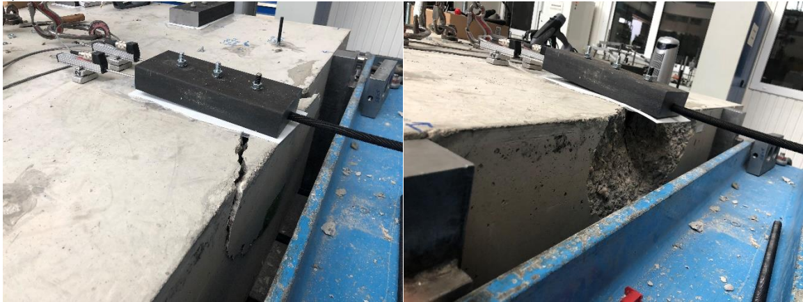
Figure 14.3. a) Load-displacement curves on 3 \times 1 anchor groups with different failure modes for the anchors reproduced from Bokor (2019) and result of the spring model; b) failure mode
