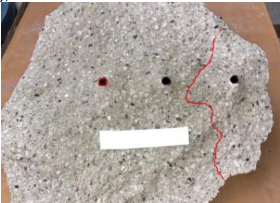
Figure 8.8. a) Load-displacement curves of test series G51R-G53; Axial anchor forces and group force in function of elapsed time for test series: b) G51R; c) G52; d) G53; Typical failure modes of test series: e) G51R; f) G52; g) G53
