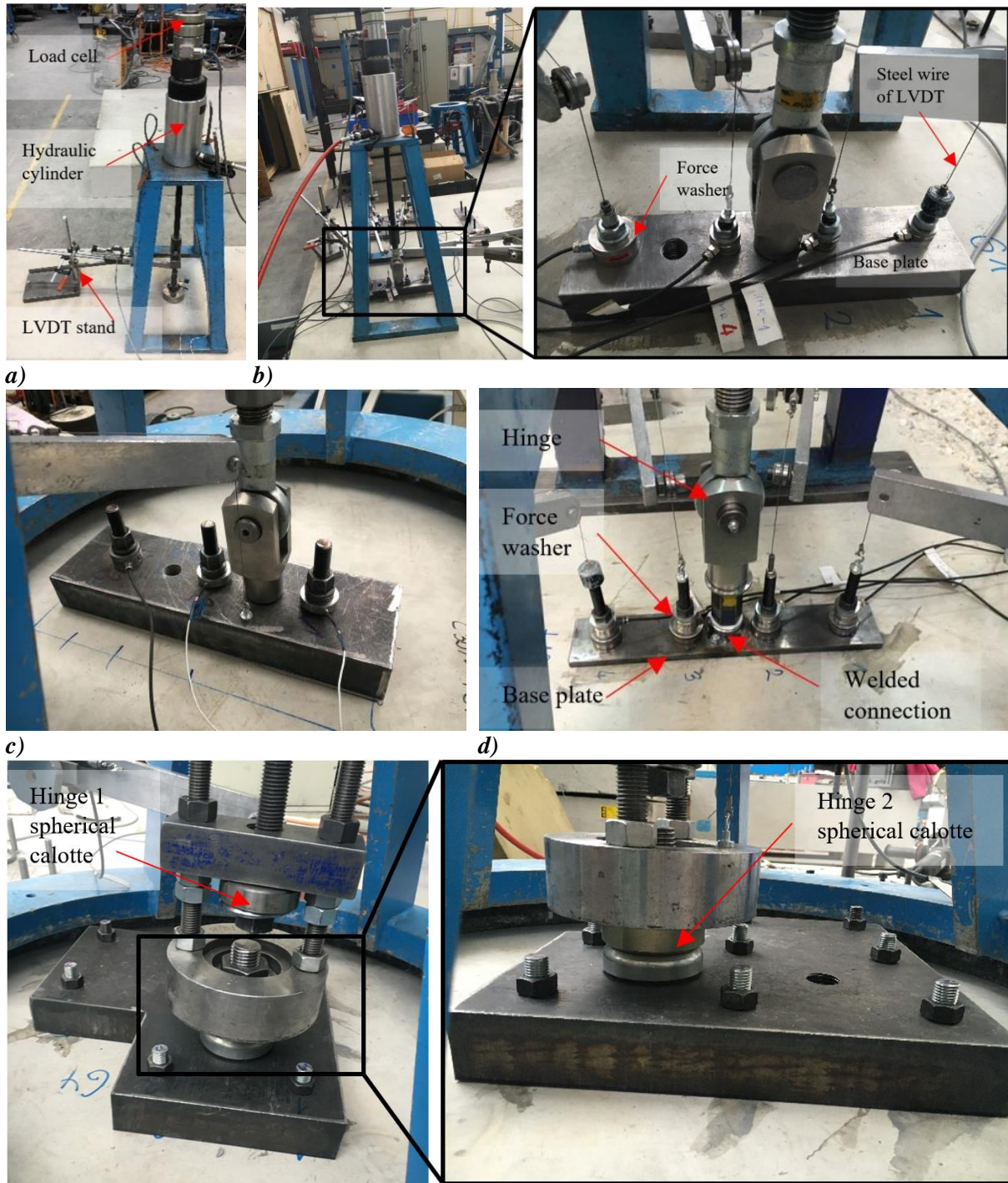
Figure 8.3. Typical test setup in uncracked concrete a) for reference tension tests on single anchors; b) for tension tests on anchor groups with stiff base plate; c) for eccentric tension tests; d) for tension tests on anchor groups with non-rigid base plate; e) for tension test on anchor groups of L-shaped configuration
