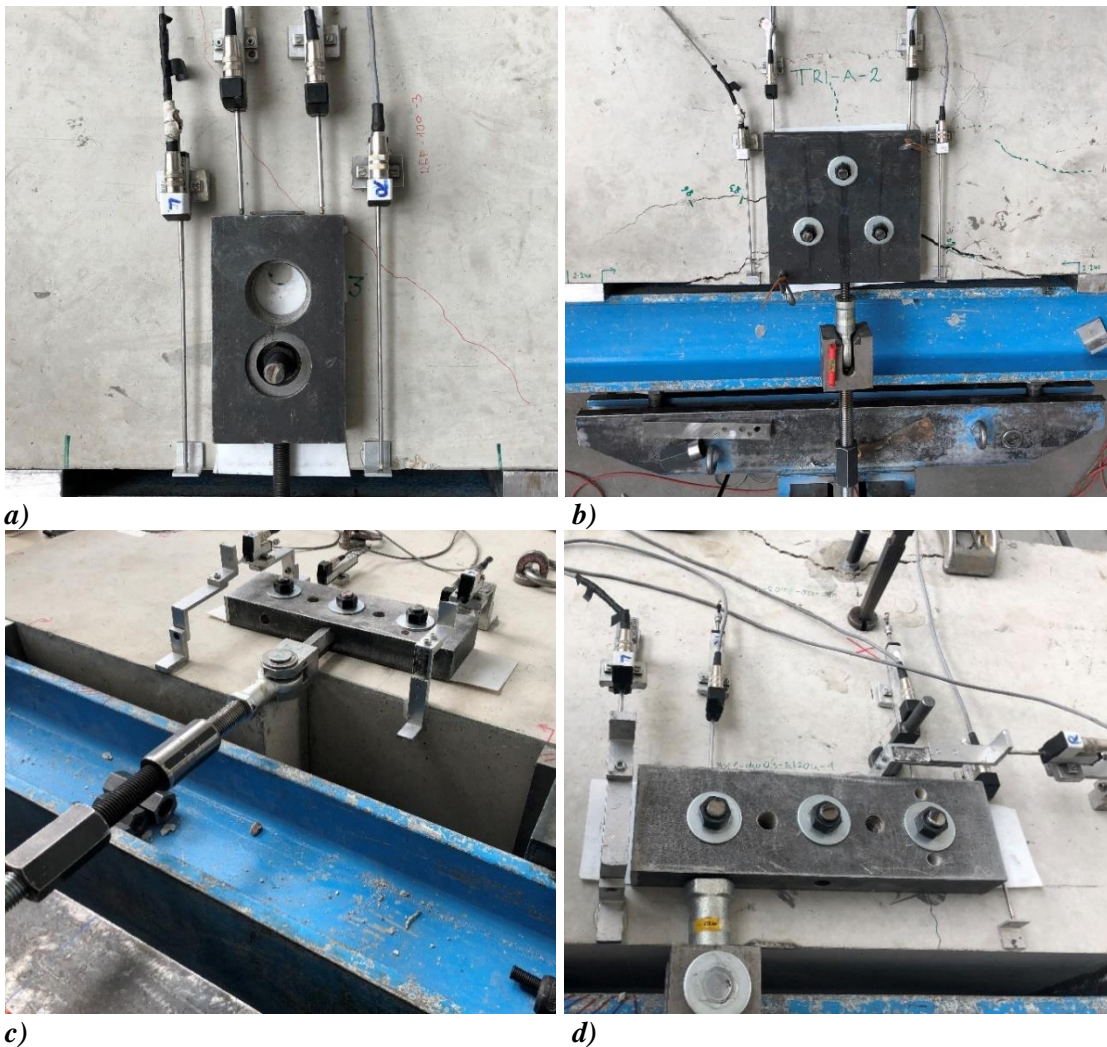
Figure 9.5. Schematic of the setup for shear loading tests – loading perpendicular to the concrete edge
