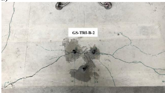
Figure 9.27. Test series with triangular configuration: a) load-displacement curves; Failure crack pattern of test: b) GS-TRI-A-1, c) GS-TRI-A-2, d) GS-TRI-A-3, e) GS-TRI-B-1, f) GS-TRI-B-2, g) GS-TRI-B-3
