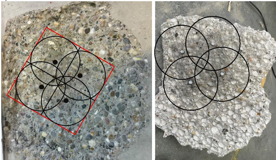
Figure 10.2. Anchor group of 2 x 2 configuration - G31R test 1: a) Load-displacement curves; b) concrete breakout surface and the corresponding breakout body
