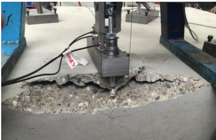
Figure 8.6. a) Load-displacement curves of test series G22 and G23; b) failure mode of series G22
