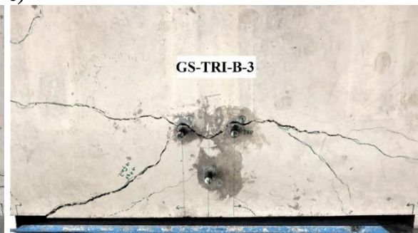
Figure 9.27. Test series with triangular configuration: a) load-displacement curves; Failure crack pattern of test: b) GS-TRI-A-1, c) GS-TRI-A-2, d) GS-TRI-A-3, e) GS-TRI-B-1, f) GS-TRI-B-2, g) GS-TRI-B-3
