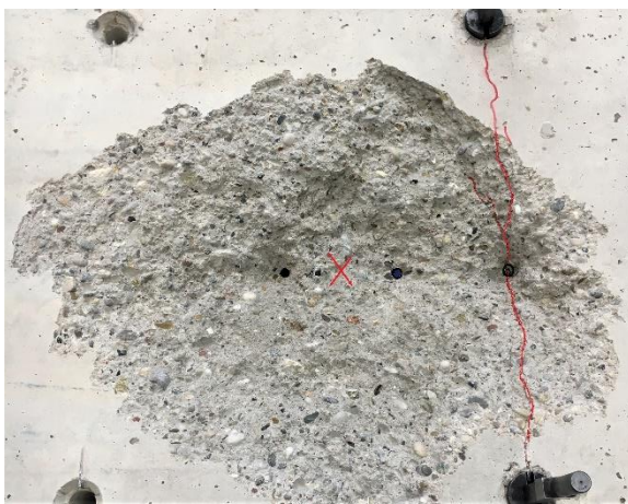
Figure 8.19. a) Load-displacement curves of test series G65, G66, G68; b) breakout body of one representative test of series G65; failure pattern of one representative test of series: c) G66, d) G68
