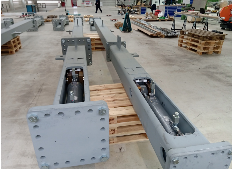
Figure 8.2: Vertical supports of the adaptive high-rise demonstrator after installation of hydraulic actuators (image by courtesy of IKTD 2 )
