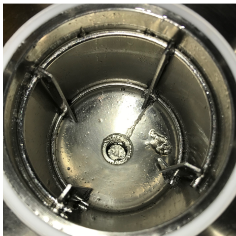
Figure 23. Fouling in the vessel of a tank reactor operated in continuous mode with a hydrodynamic residence time of 2.25 h after an experiment as described in the text and Table 1. The experiment took 29 h.
