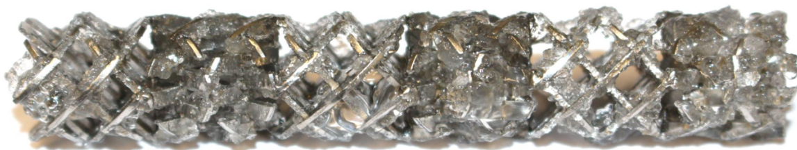
Figure 11. PVP gel fouling on a static mixer element with reduced surface roughness by slide grinding. The experiment was conducted as described in the text and Table 1 with a superficial velocity of 6\text{ mm s}^{-1} .
