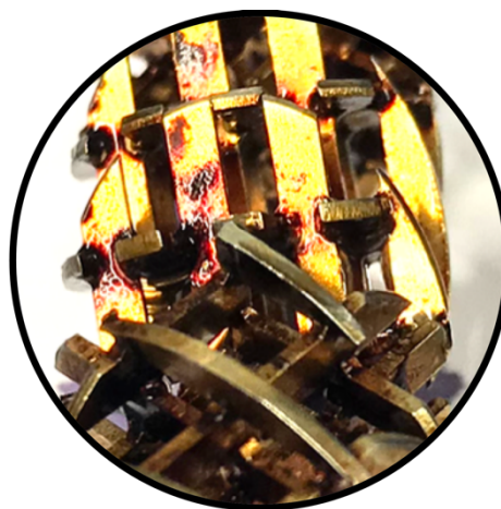
Figure 16. Dyeing (iodine solution) of a casted steel static mixer element with reduced surface roughness through slide grinding after an experiment as described in the text and Table 1 with a superficial velocity of 6 mm s -1 with subsequent water jet cleaning.
