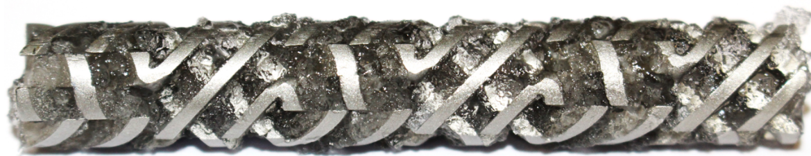
Figure 8. PVP gel fouling on a casted steel static mixer element. The experiment was conducted as described in the text and Table 1 with a superficial velocity of 6 \text{ mm s}^{-1} .
