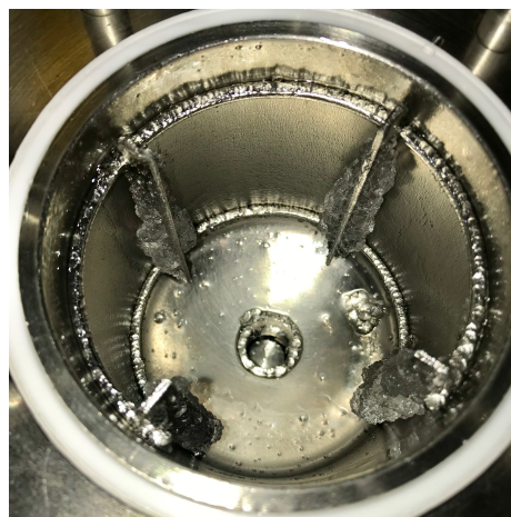
Figure 22. Fouling in the vessel of a tank reactor operated in continuous mode with a hydrodynamic residence time of 4.5 h after an experiment as described in the text and Table 1. Heavy fouling deposits were observed on metal surfaces in contact with liquid. The experiment took 56 h.
