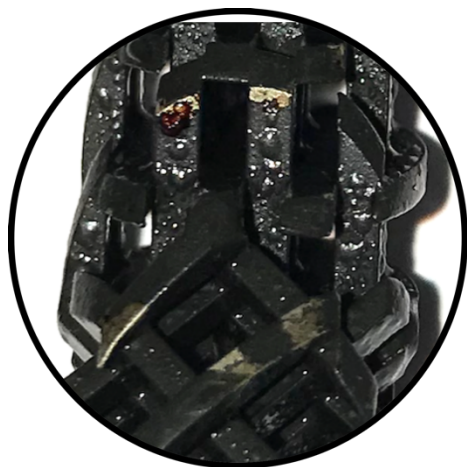
Figure 15. Dyeing (iodine solution) of a casted steel static mixer element with hydrophobic coating after an experiment as described in the text and Table 1 with a superficial velocity of 6 mm s -1 with subsequent water jet cleaning.
