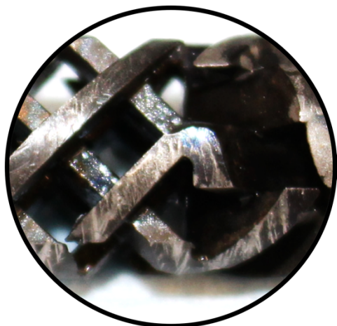
Figure 14. Effect of thermal cleaning at 600 °C on PVP gel fouling on a static mixer element. The casted steel static mixer element was subject to strong fouling in several experiments as described in the text and Table 1 with a superficial velocity of 6 mm s -1 with water jet cleaning in between (similar to Figure 12). The picture shows the same mixer element after thermal treatment in an oven and repetition of the experiment.
