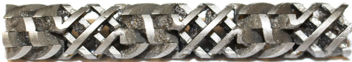
Figure 7. Initial states (5.5 h of operation) of PVP gel fouling on a casted steel static mixer element. The experiment was conducted as described in the text and Table 1 with a superficial velocity of 6 \text{ mm s}^{-1} . The direction of flow is from right to left.
