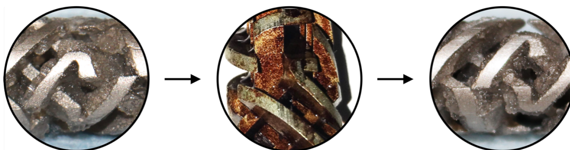
Figure 12. Effect of mechanical cleaning with water jet on PVP gel fouling on a casted steel static mixer element. Left: casted steel static mixer element after several experiments as described in the text and Table 1 with a superficial velocity of 6 \text{ mm s}^{-1} with water jet cleaning in between. Middle: same mixer element after mechanical cleaning with water jet and dyeing with iodine solution. Right: mechanically cleaned mixer element after repetition of the experiment.
