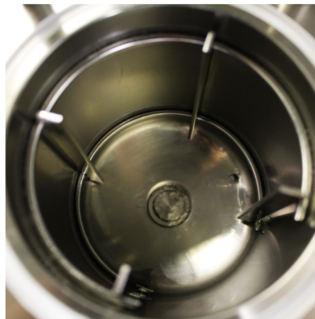
Figure 24. Fouling in the vessel of a tank reactor operated in continuous mode with a hydrodynamic residence time of 2.25 h after an experiment as described in the text and Table 1 but the feed concentration of monomer was decreased to w_M^0 = 0.1 . The experiment took 29 h.
