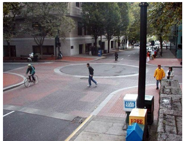
Fig. 2- 39 (below right) A raised junction combined with a small roundabout in Portland, Oregon
