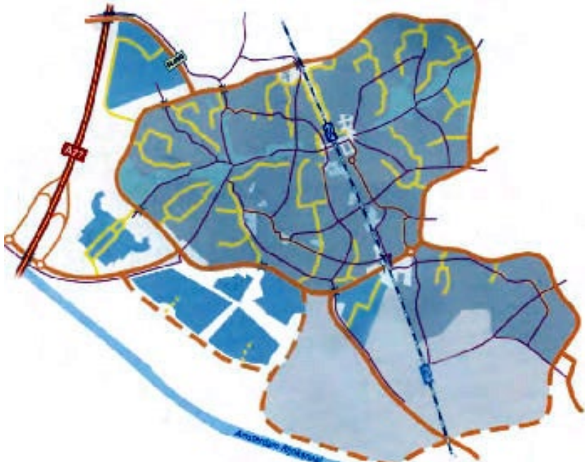
Fig. 2- 15 A schematic plan of Houten showing bicycle paths (in purple), car traffic (in yellow) and the ring road (brown) (source: redrawn from a map provided by the Municipality of Houten)
