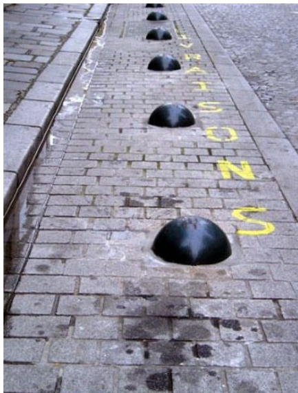
Fig. 2- 53 Devices to hinder normal cars from parking in certain locations (source: courtesy of Poutchy-Tixier)
