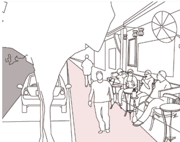
Leaving 1.2-1.5m in the fina' space for social, commercial uses, also for placing drinking fountains, and then leaving min. 1.8m for walking
