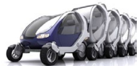
Fig. 2- 57 Stackable electric vehicles, designed by Franco Vairani & MIT Smart Cities Research team (source: Jha 2005, original photo taken by Franco Vairani, MIT Department of Architecture)
