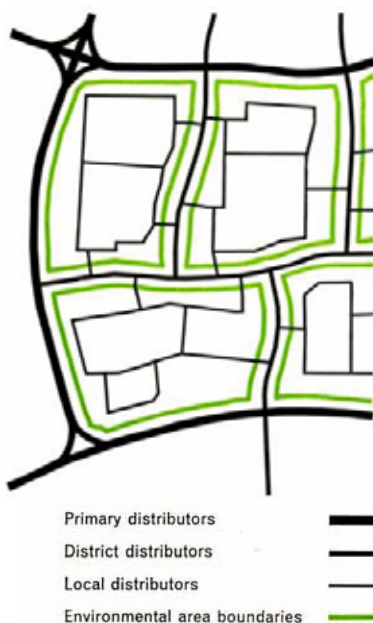
Fig. 2- 22 Buchanan's environmental areas (within the green boundary), from which extraneous traffic is banned and his devised hierarchy of traffic distributors.
